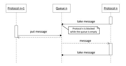
Figure 5.11.: Sequence diagram of an Activity taking a message from a queue
